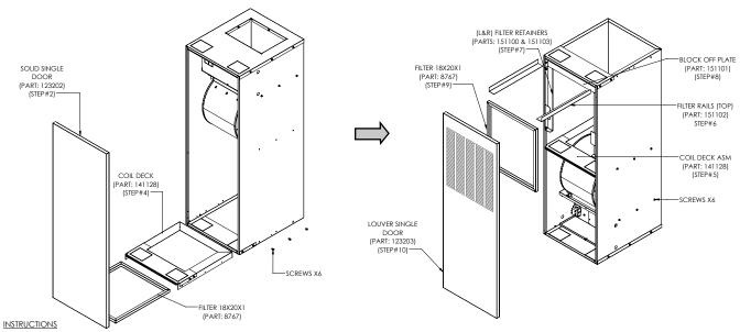
STEP 1: REMOVE THE DOOR (123202), FILTER, COIL DECK (141128)
