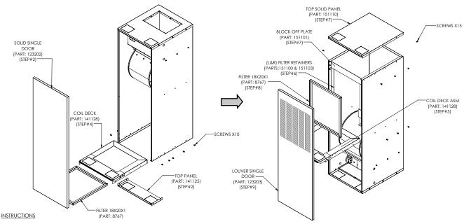
STEP 1: REMOVE THE DOOR (123202), FILTER, COIL DECK (141128) & TOP PANEL (141125) STEP 2: DISCARD THE PARTS# 123202, 141125
