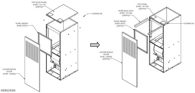
STEP 1: REMOVE THE DOOR (123203), FILTER & TOP SOLID PANEL (151110) STEP 2: DISCARD THE PART# 151110
