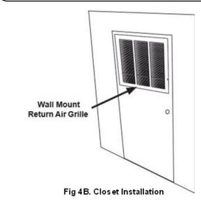
Airflow must be available to the electric furnace's return. Not doing so may cause improper heating as well as premature heating element failure.
