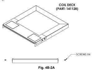
**Step 2:** Configuring the Coil Deck Assembly, extend coil assembly when in a downflow configuration (Figure 4B-2B) and collapse the assembly when in an upflow configuration (Figure 4B-2C).
