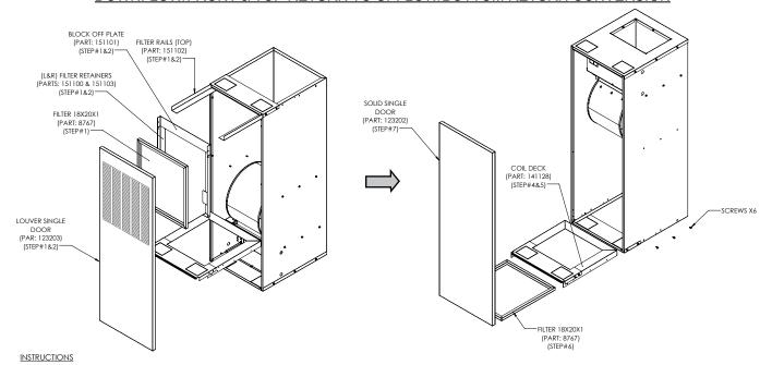
STEP 1: REMOVE THE DOOR (123203), FILTER (8767), FILTER RAILS (151100 & 151103), TOP FILTER RAILS
