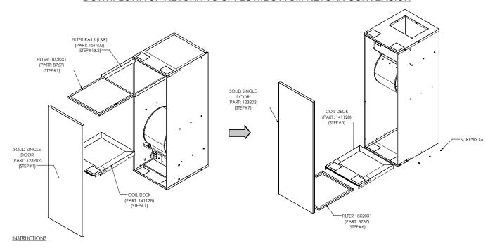
STEP 1: REMOVE THE DOOR (123202), FILTER (8767), TOP FILTER RAILS (151102) & COIL DECK (141128)
