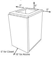
For closet installation, the return air opening can be on the front door, above the furnace casing on a wall, or on the electric door's louvered door (If applicable.)
